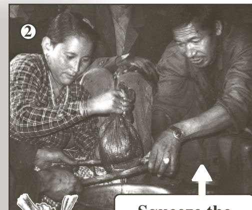
Squeeze the cooked wax in a bag between two sticks. The molten wax looks like oil.
