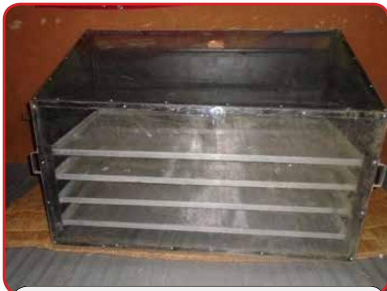
Above - a solar drier, manufactured in Surkhet, with a capacity to dry up to 10kg of fruit and vegetables. This is on its way to Humla for testing
