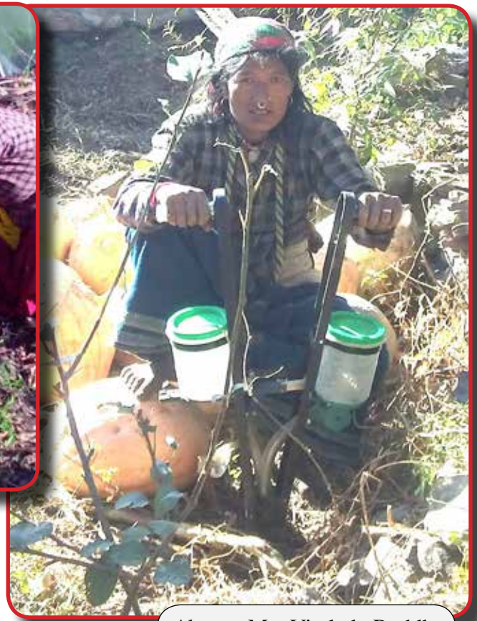
Above - Mrs Vimkala Buddha testing the jab planter, manufactured in the government's Agricultural Technology Centre in Kathmandu. The jab planter is designed to plant large seeds such as corn, beans and peas through thick mulch. The mulch has the function of retaining moisture and preventing weeds (while also contributing biomass to the soil), and so crops can be sown without tillage/ploughing disturbing the soil and its micro-life.
