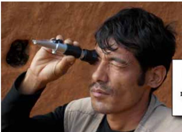
Surkhet technician and beekeeping expert Kul B. Buddha tries out the new refractometer for measuring water content in honey
